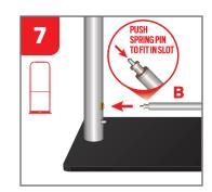
CONNECT THE LOWER HORIZONTAL BAR (B) INTO THE BRONZE HOLES NEAR THE BASE.
