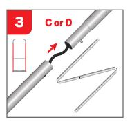
ASSEMBLE THE VERTICAL POLES (C AND D) BY ATTACHING THE THREE SEGMENTS TETHERED BY A BUNGEE CORD.
