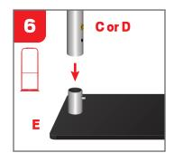
ATTACH THE ASSEMBLED TENSION BANNER STAND FRAME TO THE BASE (E).
