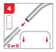
ATTACH THE VERTICAL POLES (C AND D) TO THE ASSEMBLED TOP SECTION FROM STEP 2.
